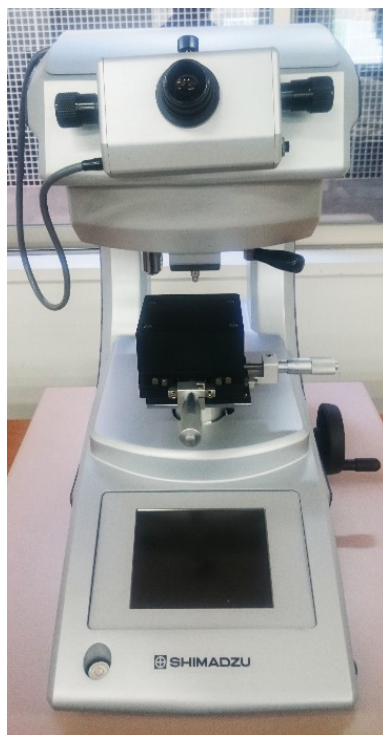
Fig.2-13 Overview of Vickers hardness apparatus
