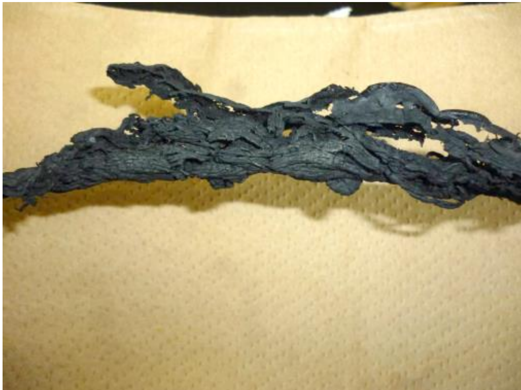
Figure 2.21.(a) Formed PVC sheathing at 55\text{ kW/m}^2 .
