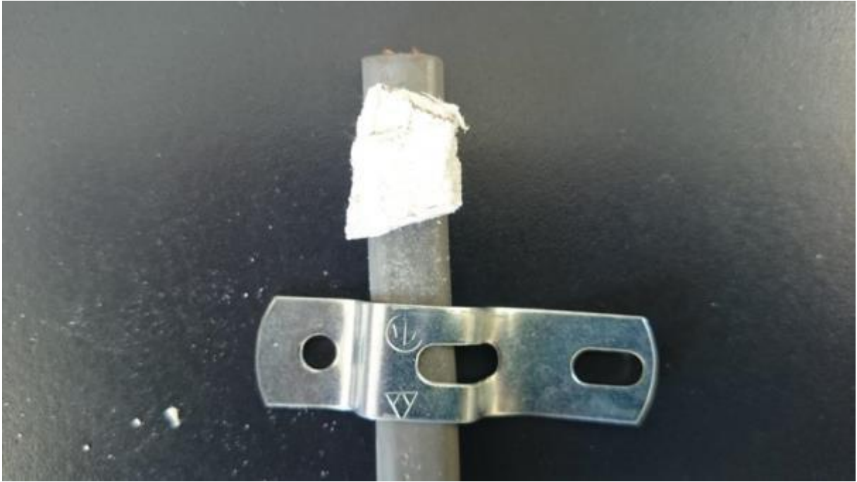
Figure 4.5.(a) Cable fixing method.
