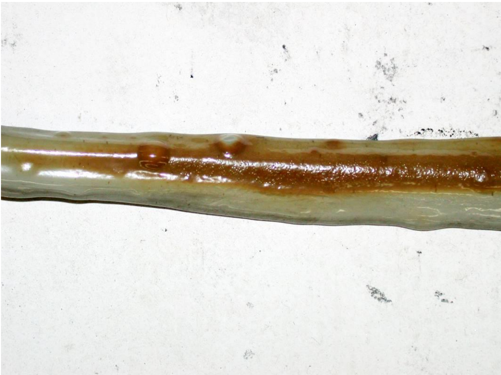
Figure 2.21.(c) Formed PVC sheathing at 10 kW/m 2 .
