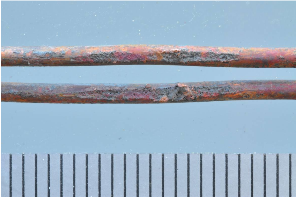
Figure 4.15.(b) Arc marks after conductor has been separated.
