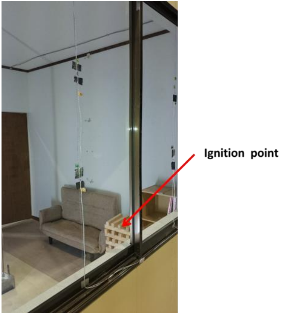
Figure 4.2. Inside the test compartment.
