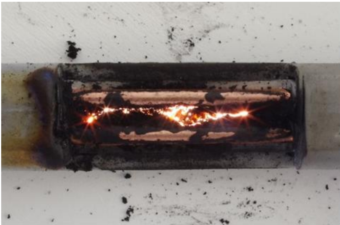
Figure 3.15. A typical occurrence during an arc through char is the spreading out of the leakage current.
