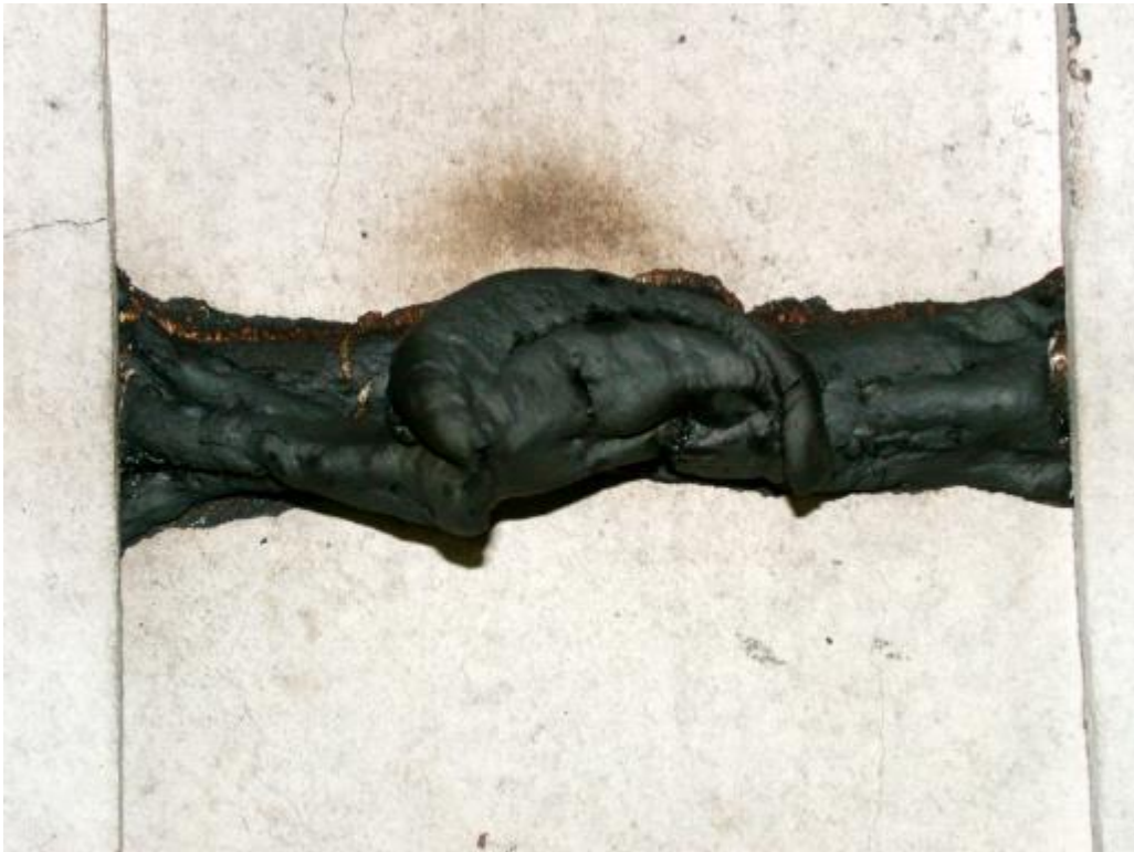
Figure 2.21.(b) Formed PVC sheathing at 20 kW/m 2 .
