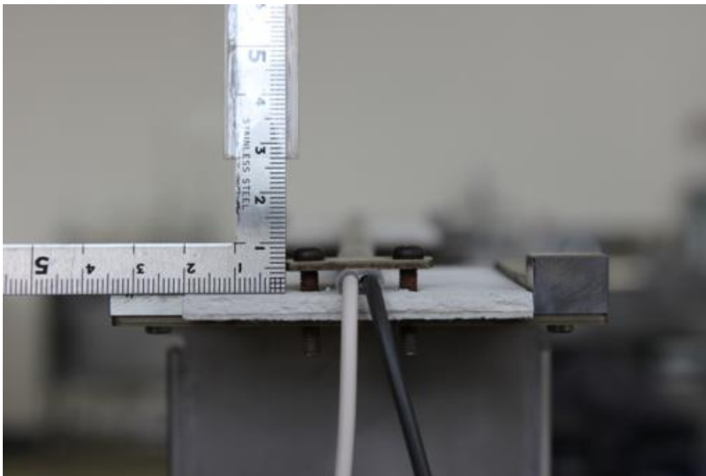
(c) The cables are fixed at a height of 4.5 mm using a torque wrench. The wrench is torqued to 25 cN·m.
