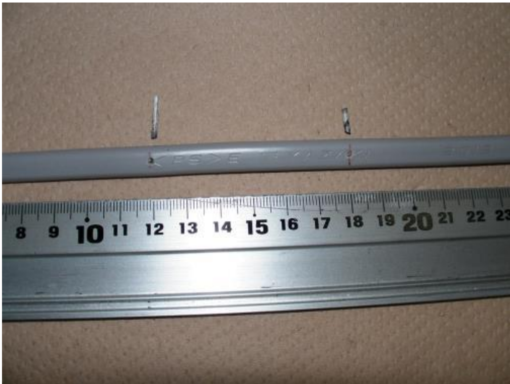
(b) In order to promote an arcing short conductors in the cable arc held apart using ceramic pins. The pins are 3 cm apart from the center of the
