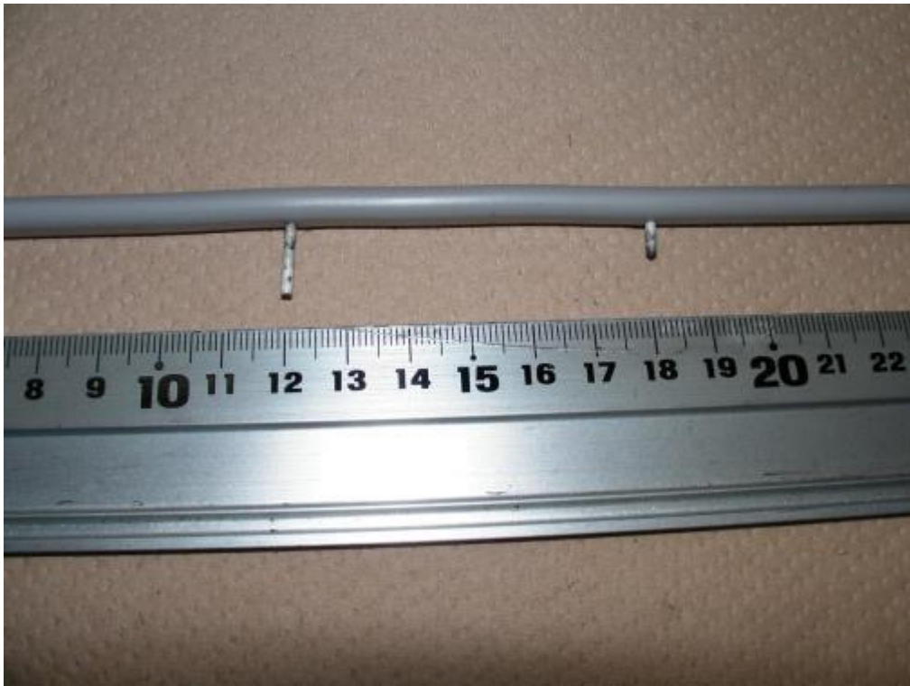
(c) Ceramic pins are inserted into the cable.
