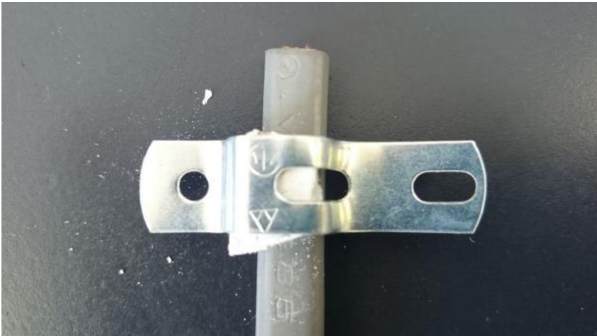
Figure 4.5.(b) Cable fixing method.
