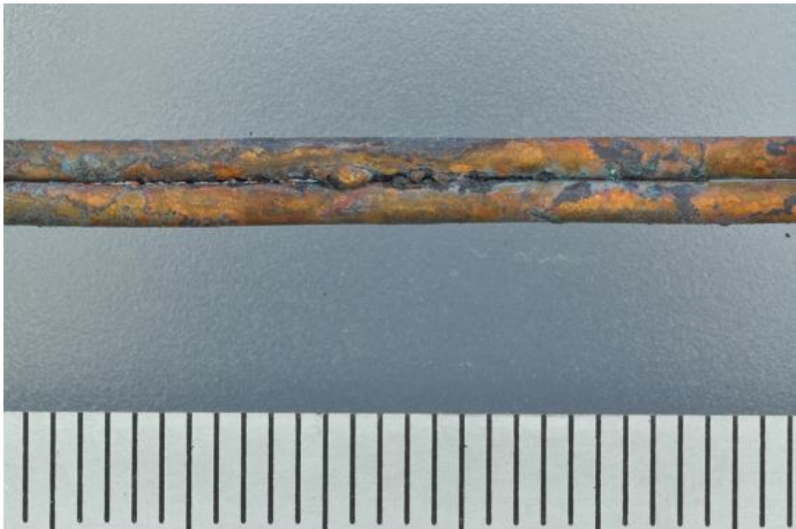
Figure 4.9.(a) Arc marks on VVF1 conductor.
